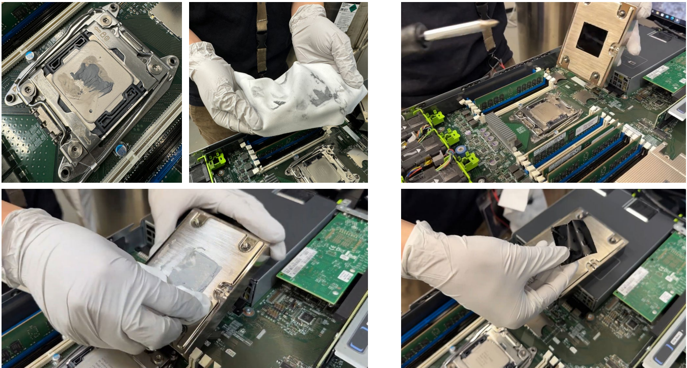
FIGURE 11: Messy thermal paste (left) vs. clean Carbice solution (right).
