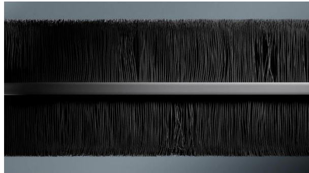
Figure 1 A 3D rendering of the cross sectional view of the vertically aligned carbon nanotubes on both sides of an Al substrate
